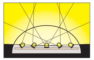
Patlite has created a revolutionary patented lighting design in which multiple LEDs project light across a broad peripheral area, ensuring equal intensity at the sides as well as the front. This design, with its side-projection technology, is a unique achievement in signal light design.
