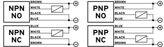
These sensors, thanks to the unpaired output circuit offer 4 output configurations (NPN-NO, NPN-NC, PNP-NO, PNP-NC) on the same model.
