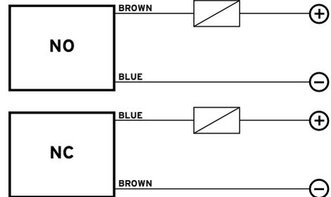
**WARNING:** The load can be connected in series to the blue wire or to the brown wire to simulate the NPN or PNP functioning logic.
