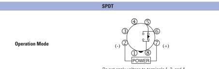
Do not apply voltage to terminals 1, 3, and 4. 2 - 7 (8p) 5 - 8 (8p) (NC) Delayed Contact **ON-Delay** (NO) POWER Indicator OUT 100 70 50 30 20 24V DC Resistive Load 120V AC Resistive Load 10 240V AC Resistive Load
